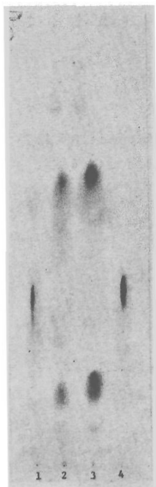
Figure 2. (1) Synthetic VIP, 80 \mu\text{g} ; (2) synthetic VIP, 80 \mu\text{g} , degraded with kallikrein; (3) natural VIP, 80 \mu\text{g} , degraded with kallikrein; (4) natural VIP, 80 \mu\text{g} . Electrophoresis conditions: 90 min at 50 V cm in pyridine-acetic acid-water (300:11.5:2700 4 v/v) at pH 6.4 using Whatman 3MM paper. Some loss of the synthetic peptide, probably due to aggregation, occurred in these experiments.
